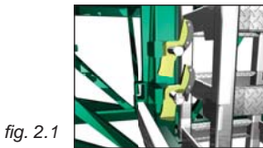
fig. 2.1 Safety hooks in normal working position
