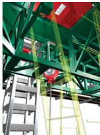
Tie a lifeline with a rope grab or a self-retracting lifeline to the designated tie point under the motorized unit
